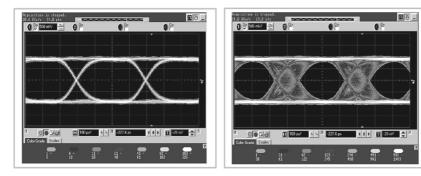
The difference between a clean signal and a signal with jitter
